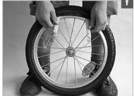
Stick the valve of the inner tube through the hole in the rim. Inflate the inner tube slightly so that it becomes round and push it into the tyre all the way round. Make sure not to leave any folds in the inner tube.
