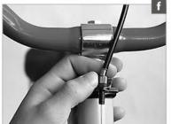
To adjust the brakes, unscrew the knurled lock ring located at the point where the brake cable enters the brake lever on the handlebar (f). Unscrew the knurled, slotted adjusting bolt by a few turns.
